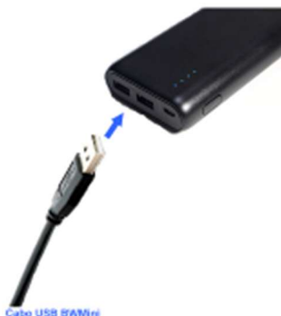
BWMini USB cable connection to battery backup
